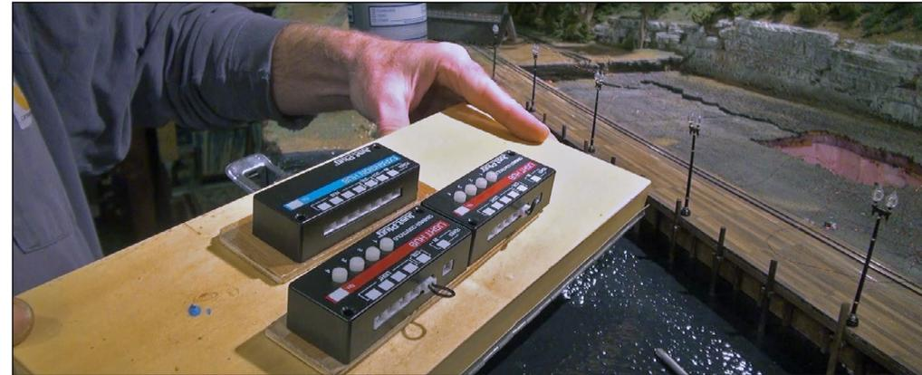
14. I used Gorilla Glue to attach two light hubs side by side in a piece of plywood. The expansion hub was also attached to its own piece of 1/4-inch oak plywood. I set this aside for 30 minutes until the glue cured.
