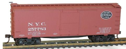
Accurail's newest body style is a group of 36-foot double-sheathed wood boxcars with various ends, doors and underframes. This New York Central car has Murphy steel ends, National wood doors and a fish belly steel underframe. All variations of the car are available painted in oxide red or mineral red and decorated with data only.
