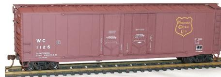
This Wisconsin Central 50-foot double plug-door steel boxcar is based on a full-size car that was rebuilt in 1983.
