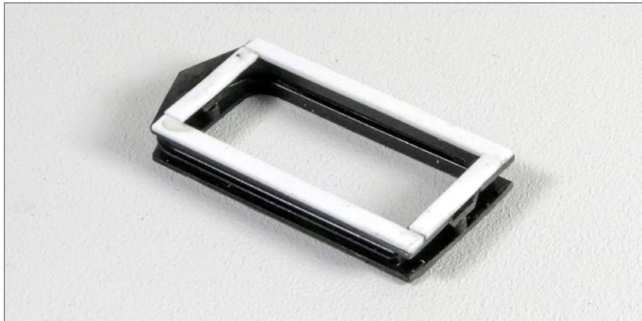
19. The diaphragm for the plastic end is modified with styrene strip spacers so as to not interfere with the roof overhang.
