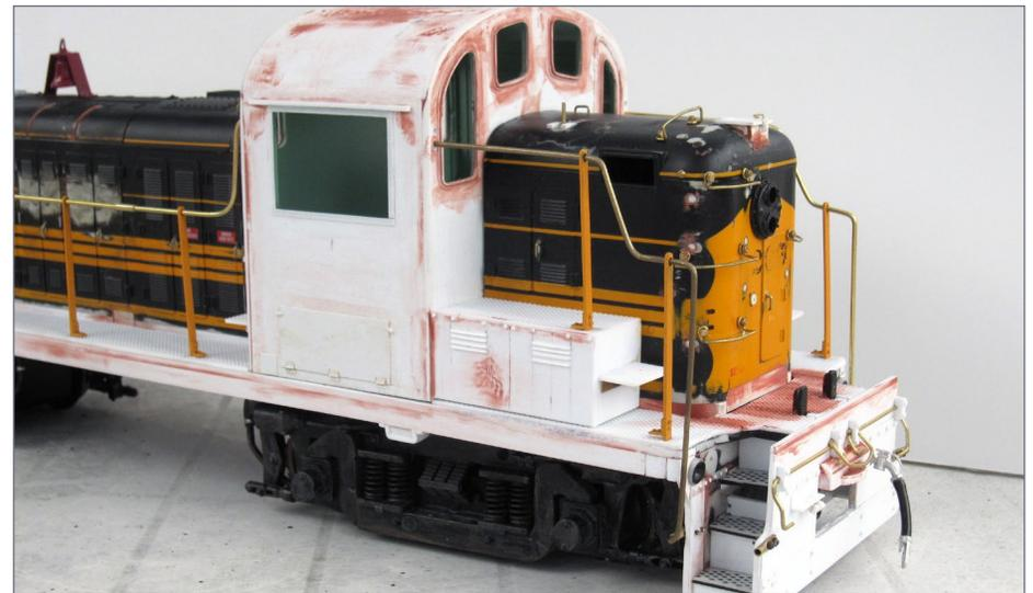
7. The RS-3 was extensively rebuilt, with a new cab, deck, pilots, handrails, and other details..
