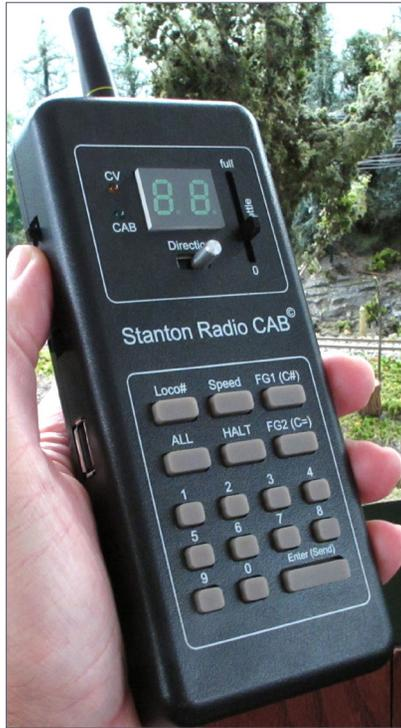
The S-CAB system operates on the 916.48 MHz frequency common to Linx boards. This makes for compatibility between the S-CAB system and others. For example the controller function could be from either an S-CAB Throttle or a TVD DRS1 transmitter. A CVP T5000 cab will work as well, using its channel 16 setting. Again, there is the interference issue with this frequency. However, the S-CAB
