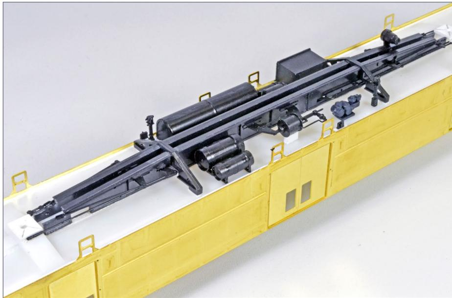
11. Underbody details are mounted to the underbody. After assembly, I discovered that the twin air tanks in the foreground should have been mounted closer to the brake cylinder, and a second battery box installed next to the cross brace, mirroring the battery box on the other side. *C'est la vie!*
