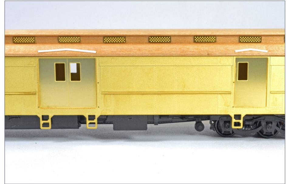
16. Drip strips are formed from styrene strip, and glued to the roof above each baggage door.
