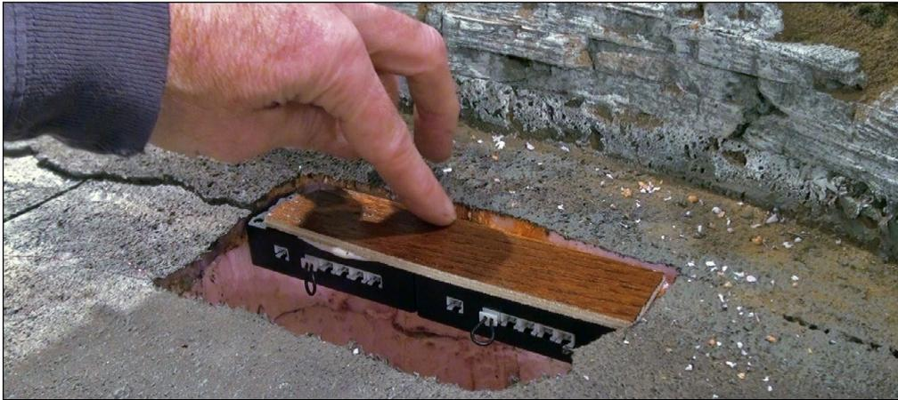
15. The two light hubs will be glued flush in the foam facing down so I will have access to the potentiometers with a long screwdriver when it comes time to adjust the lights' brightness.
