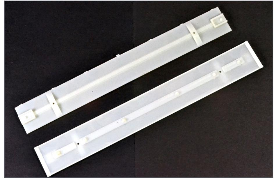
3. The floor is modified by converting the coupler boxes into mounting pads, and extending the floor's width and length.
